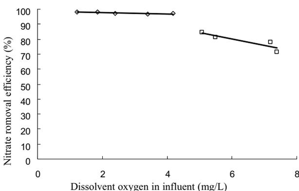
Fig. 5 Effect of dissolved oxygen on denitrification experiment using rice husk as carbon source and physical support.
