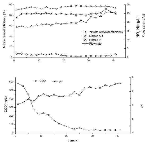
Fig. 2. Nitrate removal efficiency of the system and change of COD (mg/L) and pH according to time (d) in the effluent of a reactor packed with rice husk as physical substrate as well as sole carbon source (Temperature 29-30°C; Flow rate 16-23L/d).
