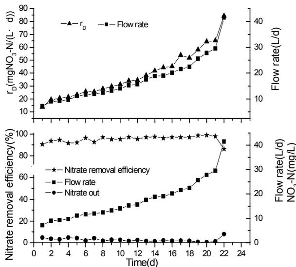
Fig. 3. Effect of flow rate (from 7.2L/d-41.0L/d) on denitrification rate and nitrate removal efficiency in a reactor packed with rice husk.
