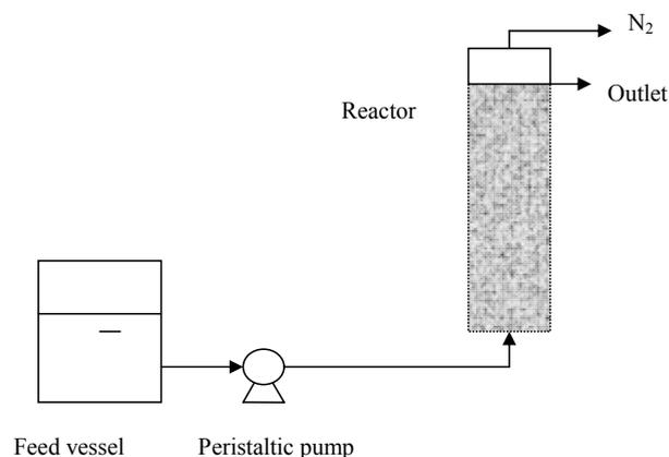
Fig. 1. Schematic of a laboratory-scale experiment.
