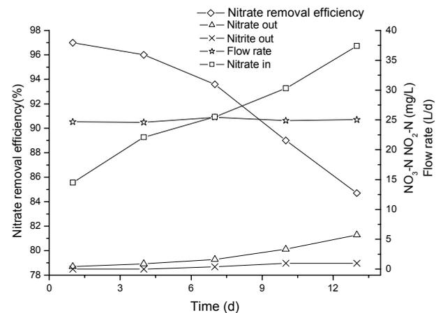
Fig. 4. Effect of nitrate loading (from 15mgNL<sup>-1</sup>-40 mgNL<sup>-1</sup>) on nitrate removal efficiency in a reactor packed with rice husk.
